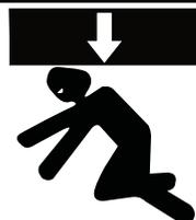
To avoid crushing and related injuries: **NEVER** work on, under or around a load supported only by a jack. Immediately transfer the load to an appropriate work station.
